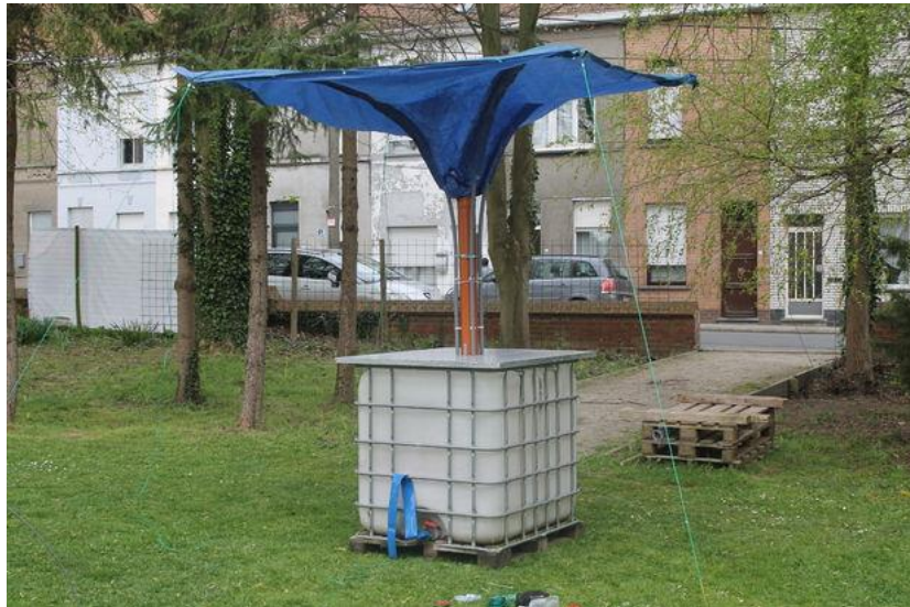
Figure 17: An Example Rainwater Collection Mechanism
